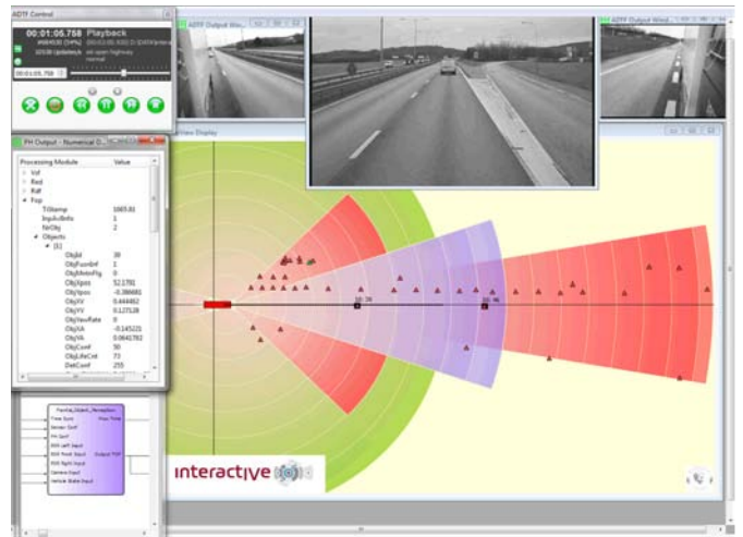
Picture 05: Output of the Frontal Object Perception Module from Volvo Group demonstrator.
