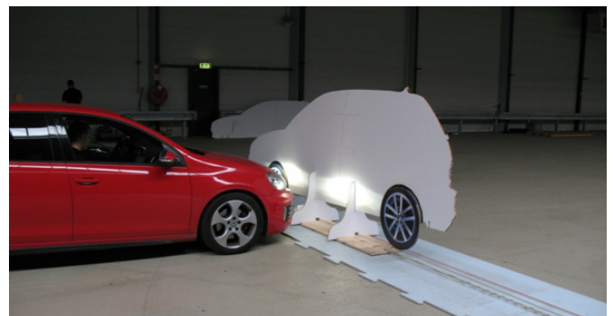
Picture 02: Collision mitigation function decelerates the vehicle before crashing into intersecting object.
