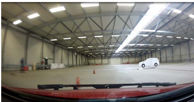
Picture 01: Testing collision mitigation at TNO test site. Intersecting object scenario from the driver’s perspective.
