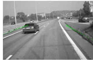
Picture 03: Snapshot of the road edge detection module from Volvo Group.
