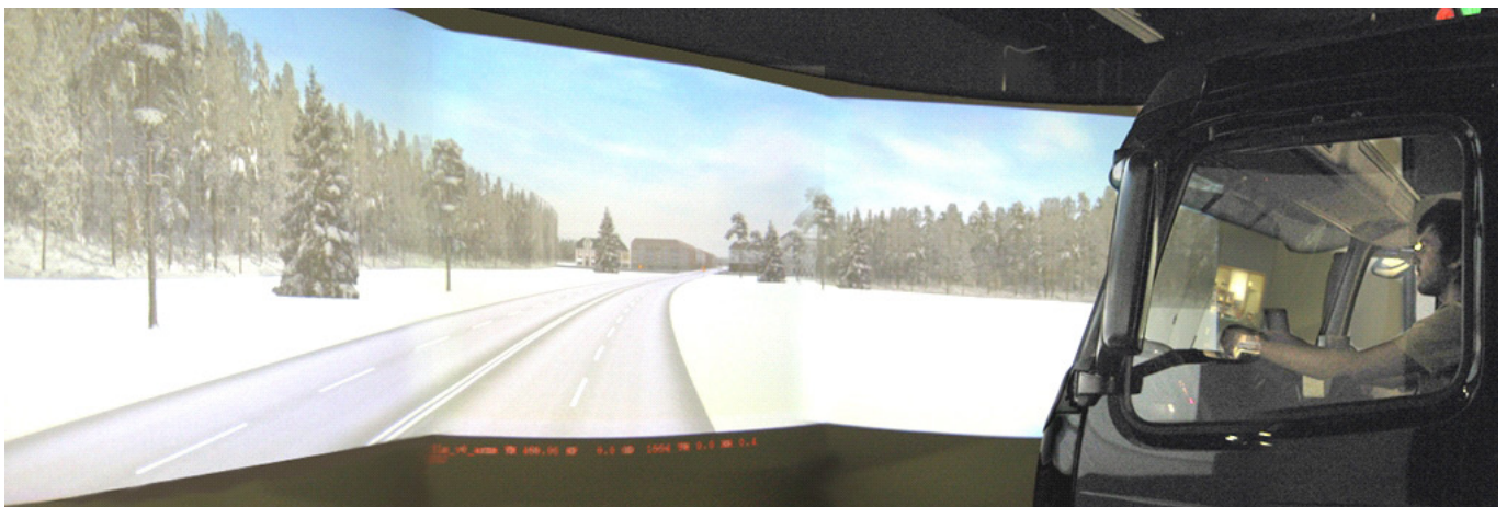
The fixed base truck driving simulator of Volvo Technology will be used for tests in interactive.
