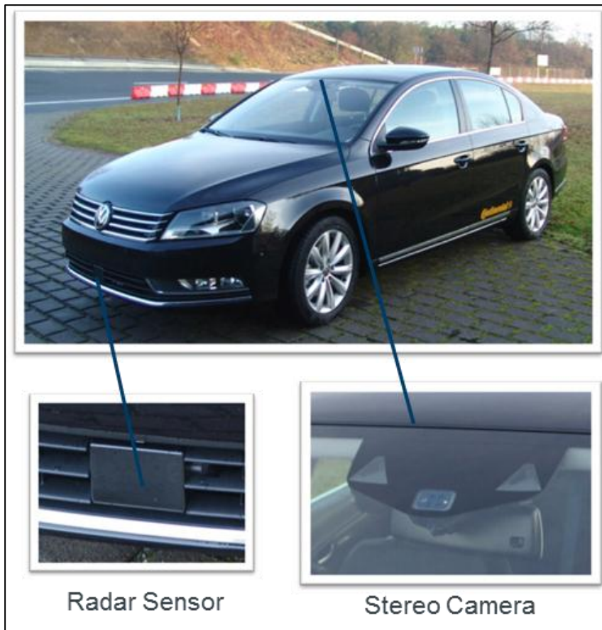
Figure 49: CONTIT demonstrator vehicle on VW Passat, with sensor system
