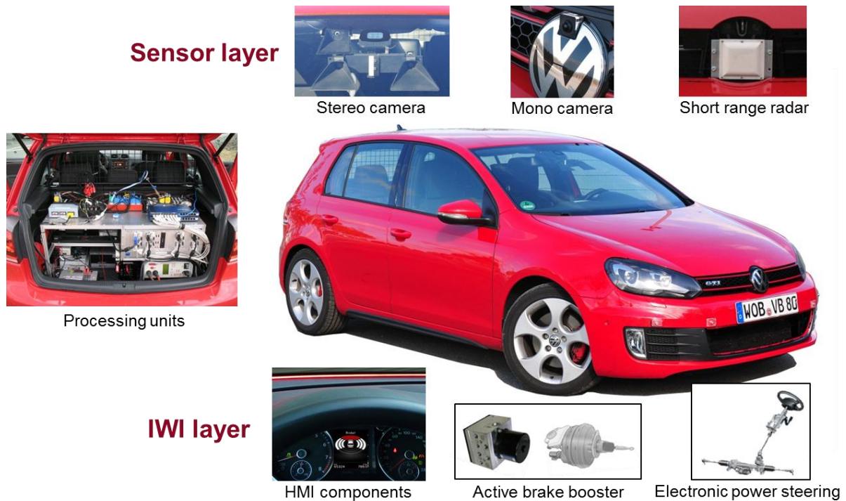
Figure 48: VW demonstrator vehicle on Golf VI GTI, with sensors and HMI components
