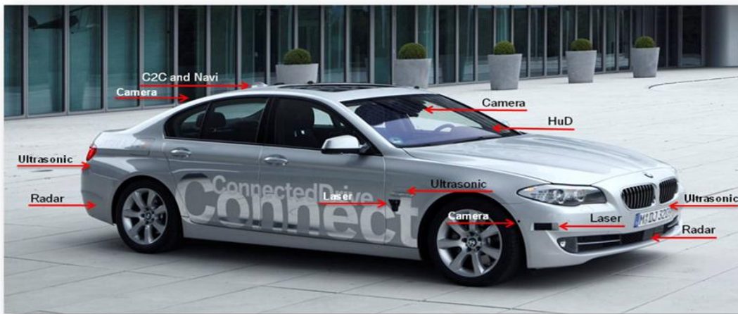
Figure 34: BMW demonstrator vehicle on i535 with the sensor system
