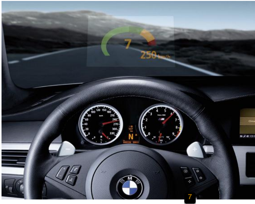
Figure 38: enhanced Dynamic Pass Predictor and head-up display
