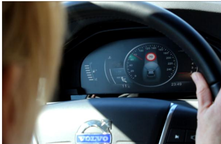
Figure 33: Full graphics cluster on the VCC demonstrator vehicle
