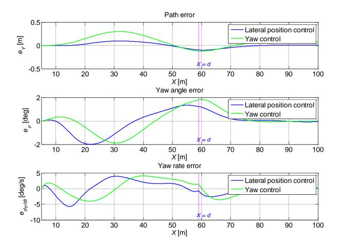
It is also tested with discrete input with update rate of 10 Hz; the controller demands new steering wheel angle every 0.1 second.
