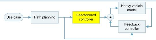
Feedforward control: steady state bicycle model is used to calculate steering inputs:
